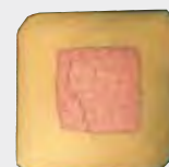
Micrograph of a square crimp
